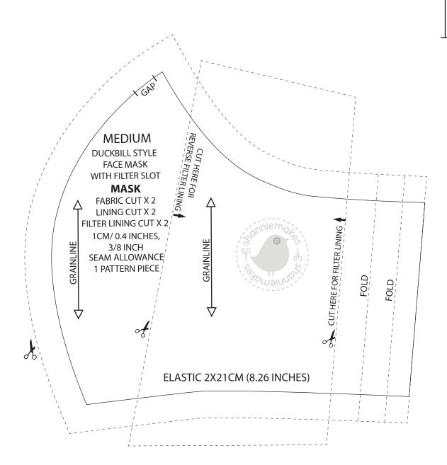
Print twice. 1 for the mask pattern, and 1 for the filter lining slot.
